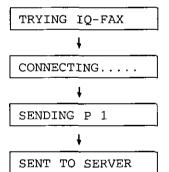
If the number you dialed is out of the FaxSav network service area, the unit will show the following messages and send the fax directly over the telephone line.
